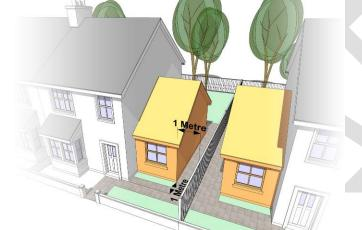
Side extensions should be set back no less than 1 metre from the front elevation of the original dwelling and no less than 1 metre from the joint/facing boundary
