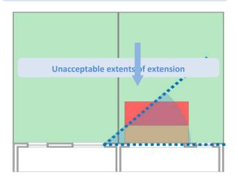
Illustration showing how the 45 degree rule will be applied in the case of two-storey/first floor rear extensions
