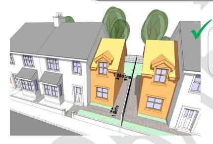
Side extensions should be set back no less than 1 metre from the front elevation of the original dwelling and no less than 1 metre from the joint/facing boundary. This is particularly important where there is the possibility of a terracing effect being created
